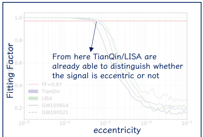
FIG. 2: The fitting factor between a noncentric template bank and a signal with different eccentricities. The blue(green) lines denote the banks of TianQin(LISA), the solid(dashed) lines correspond to the banks of a GW150914-like(GW190521-like) scenario.
